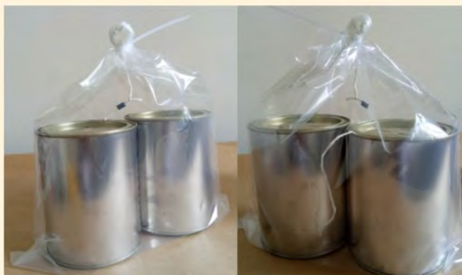
Figure 1. Schematic representation of the experimental setup for cross-contamination tests. A full-size nylon bag (12"x18") containing two 1L volume unlined metal cans with activated charcoal strips.
