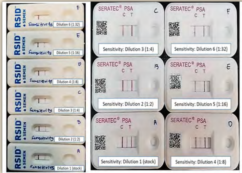
Figure 1. Sensitivity of RSID™-Semen and SERATEC® PSA Semiquant of semen extract.
